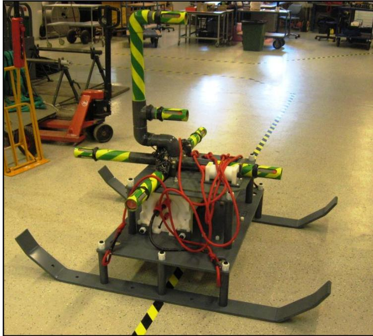
Figure 5. The sensors mounted on a sledge. This unit will be deployed on to the seabed and connected with a sensor cable to the “dry” electronics that will be situated on either the ship, or the RIB.
