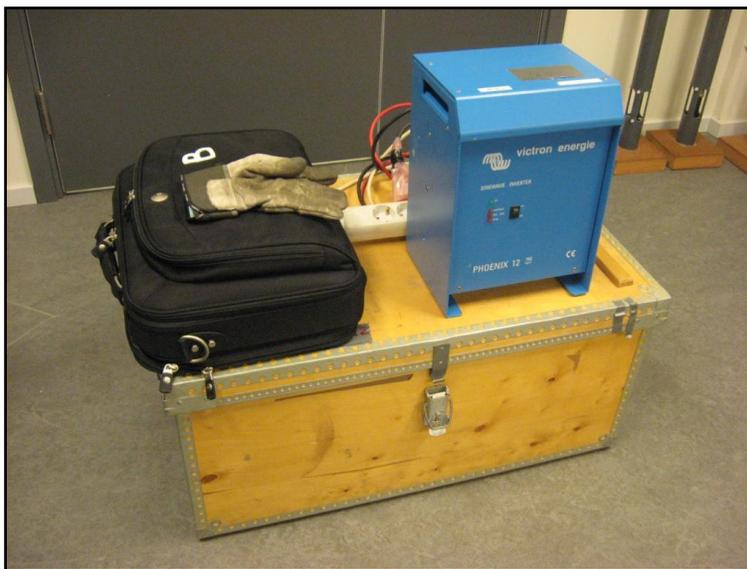
Figure 7. The wooden box that contains the electronics unit and recording instruments. Missing in the picture is the cable, which connects the “dry electronic” and the sub-surface sledge shown in Fig. 5.
