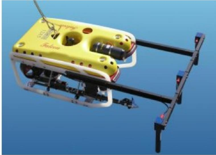
Figure 3. URI Sabb Falcon ROV and Meridian Ocean Services Innovatum 3 cable and pipeline tracker.
